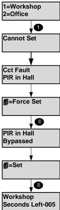
After the setting fault(s) is displayed the force set option may be presented (if programmed by the installation engineer). The force set option will attempt to automatically bypass all faults. The circuit(s) with the fault must be programmed by the engineer to allow bypass.
