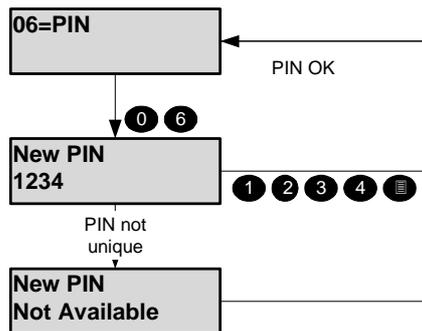
If another user on the system already uses the chosen PIN code then that user will be alerted when next logging on to the system. The user whose PIN is known must change PIN code to avoid seeing the warning message on every log on.
