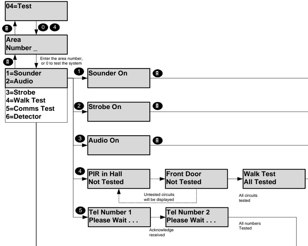
The panel records all activations from sensors during the unset period. When walk test is selected the panel will display all circuits which have not alarmed since the panel was last unset. If all circuits are to be tested then select walk test, then press the  $\chi$  button and select walk test a second time. When the panel exits walk test mode, either manually or automatically at the end of the test time then:
